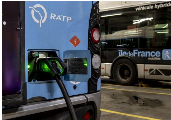
RATP bus charging at depot (Source : RATP group)
