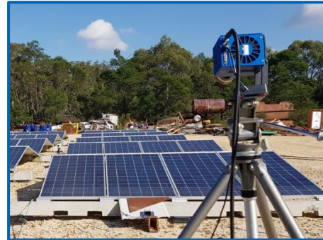
Outdoor PL imaging of PV modules
