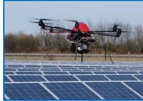
Drone-mounted IR & EL imaging of PV modules & arrays
